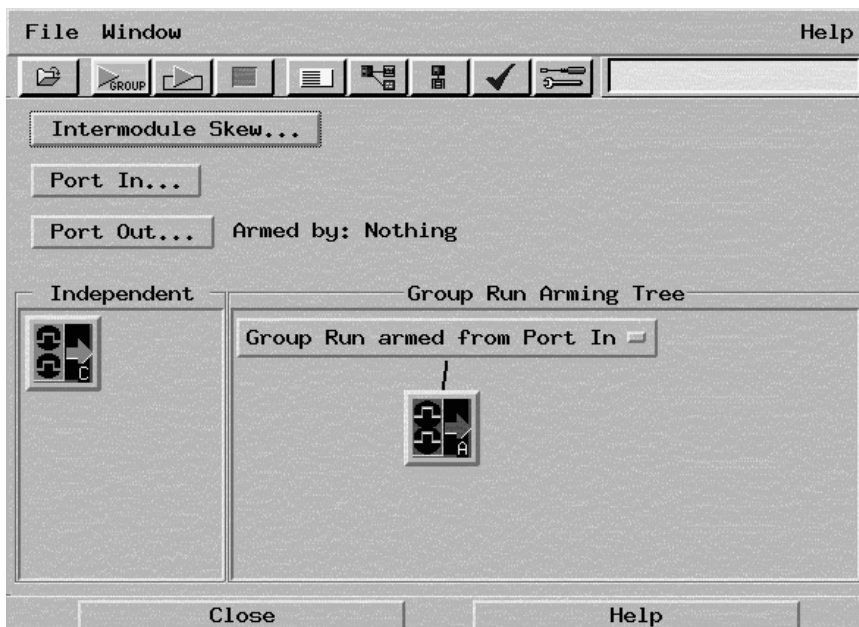
Figure 15. Setting up the 167xx analysis module to arm from Port In
